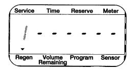
2. When the first cycle step is reached, a #1 will turn on to indicate the current regeneration cycle step.
