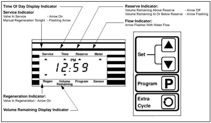
13. Whenever the valve returns to the Service Position normal operation is resumed. In normal operation the Time Of Day, and if flow meter equipped, Volume Remaining Displays alternate being viewed. Set the Time Of Day Display by depressing the Up or Down Set Button, to the correct time.
